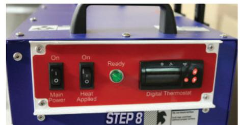
You are now ready to turn the power switch and fan switch on. Run equipment until temperature reaches 135-140 degrees and hold this temperature for 3 more hours. After this process, turn the heater coils off and let fan run for 15 minutes then turn fan off and break down equipment. **DO NOT CHANGE THERMOSTAT OR YOUR WARRANTY WILL BE VOID.**
