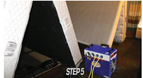
Place the BBHD-12 unit in the center of the room with the airflow blowing toward the headboard wall.
